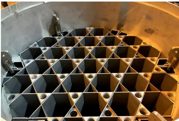
Top View of the Double Wall Multi-Purpose Canister (MPC-31) Containing Holtec-Patented METAMIC-HT Neutron Absorber for Storing and Transporting VVER Fuel
