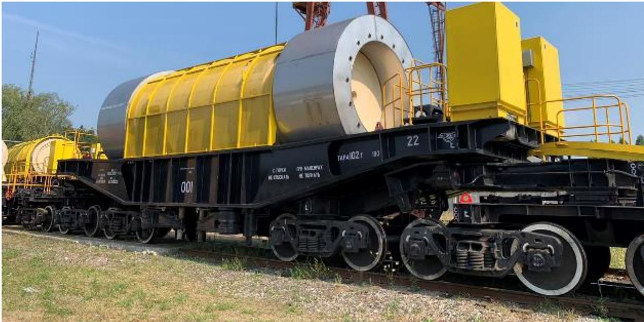
*Rivne NPP: HI-STAR 190 Transport Cask with Impact Limiters on the Specially-Designed Holtec-Supplied Rail Car*
