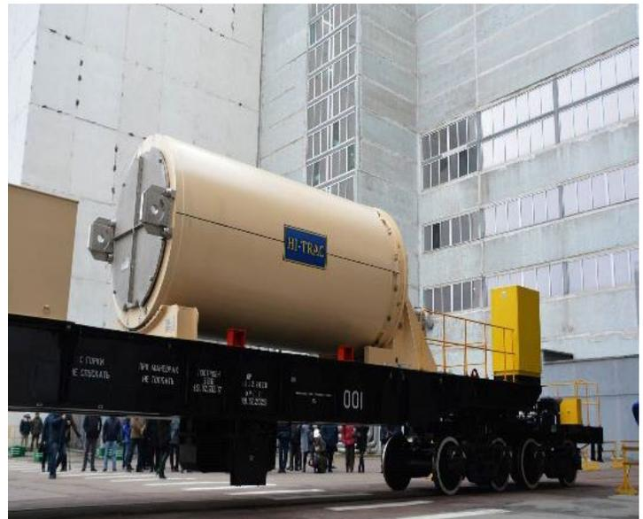
Rivne NPP: HI-TRAC 190 Transfer Cask on the Holtec-Supplied Rail Car
