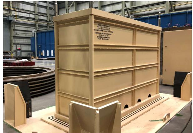
**Disposal Liner on Pool Alignment Fixture
