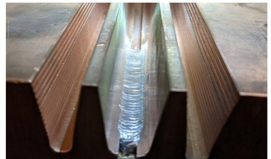
*Full Scale Mockup of Copper Weld Joint for the HI-STAR 80 with Single Pass Hybrid Arc Laser*
