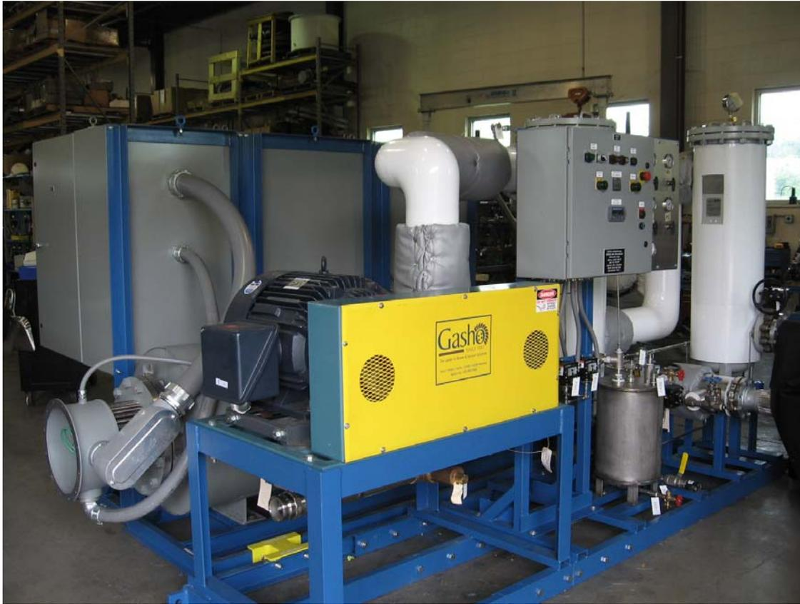
**Holtec FGD Prototype System for Chernobyl Dry Storage Project**
