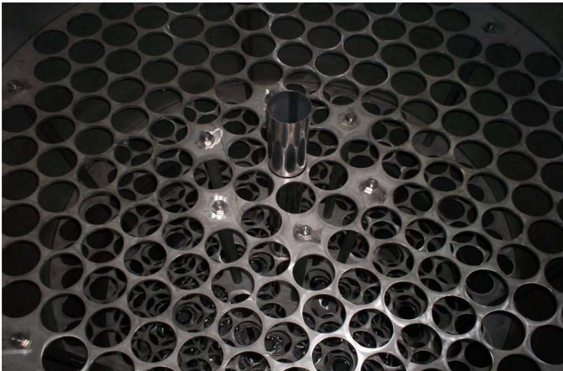
**Overhead View of Double Wall Canister/Basket Assembly**
