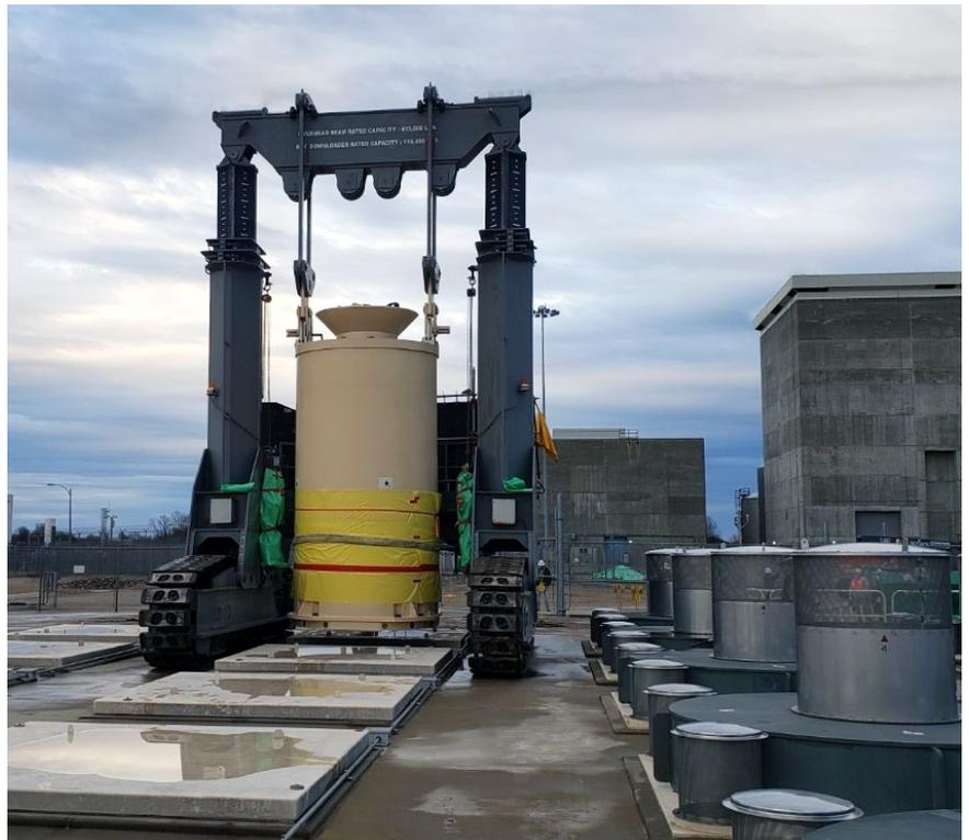
*Holtec's 1,500<sup>th</sup> Canister Being Positioned to be Safely Placed into the HI-STORM UMAX System at Ameren Missouri's Callaway Energy Center*
