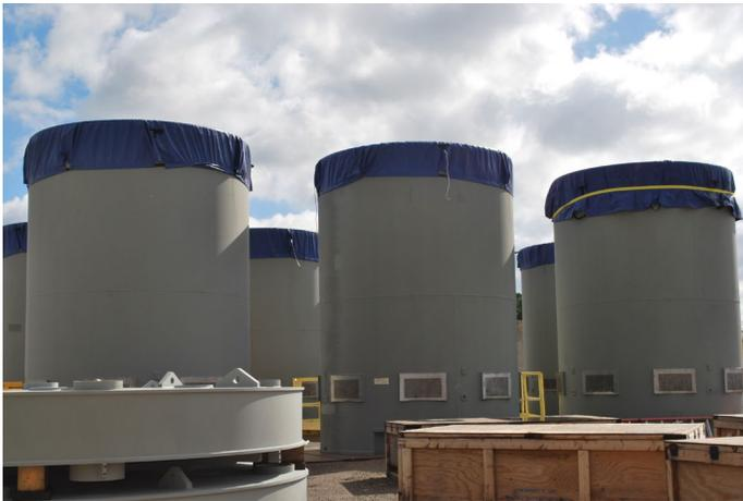
*Empty HI-STORM FW Dry Storage Overpacks to be Used for the Oyster Creek Spent Fuel Loading Campaign*
