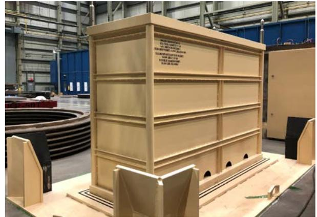
**Disposal Liner on Pool Alignment Fixture
