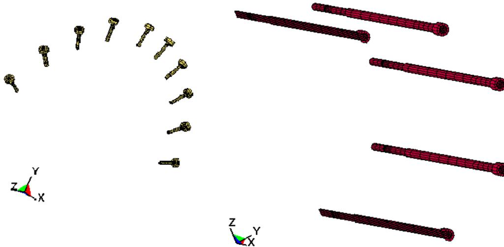
Figure 2: LS-DYNA Model of Impact Limiter Attachment Bolts
