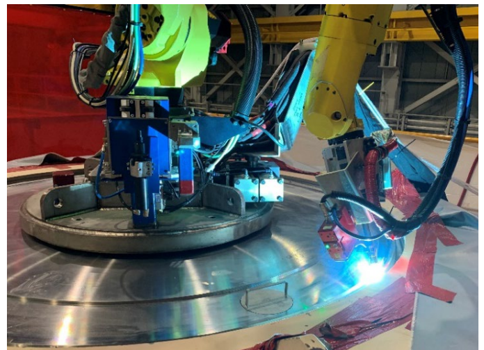
HI-BRIAN Welding the Lid to the Shell of an MPC-89
