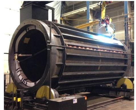
*Robotic Welding of HI-STAR Transportation Cask at Holtec Manufacturing Division in Turtle Creek, PA*
