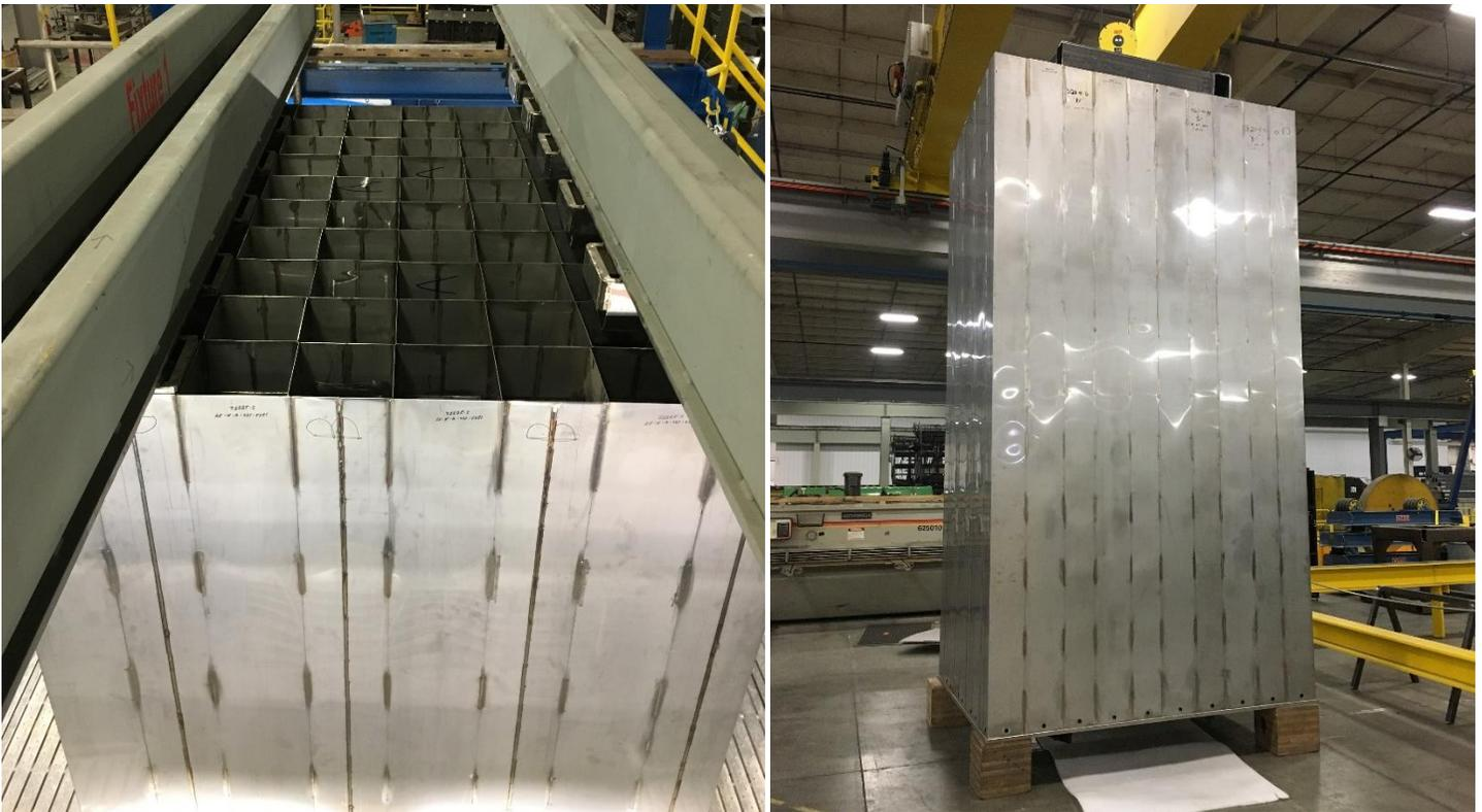
*Spent Fuel Storage Racks Fabricated for Duke Energy's Harris Nuclear Plant at Holtec's Orrvilon Manufacturing Division, in Orrville, OH*
