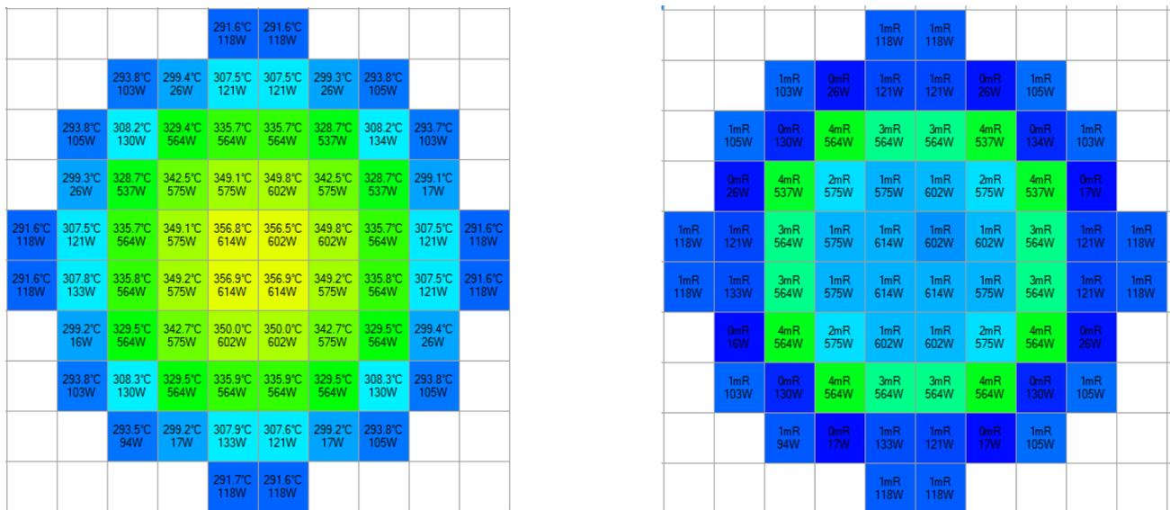
**Figure 3. Estimated fuel peak cladding temperatures (PCT) and estimated per-assembly surface dose contribution for a sample cask.**
