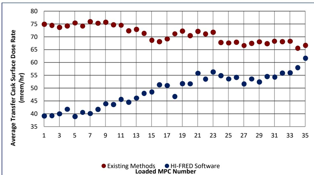
**Figure 1. Comparison of projected surface dose rates produced by traditional methods or through use of HI-FRED.**
