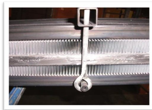
CYCLIC FATIGUE TESTING OF HI-MAX TUBE
