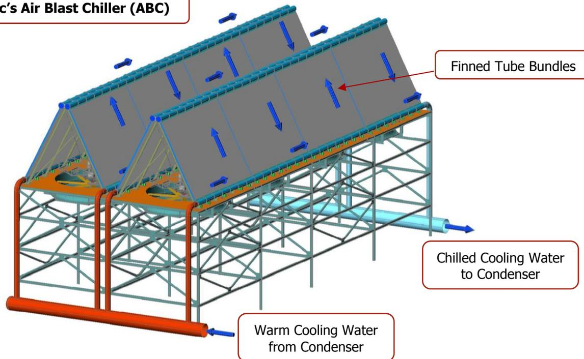
Note: Arrows indicate water flow. Horizontal arrows are top/bottom header flows and angled arrows depict multipass water flows in the finned tube bundles.
