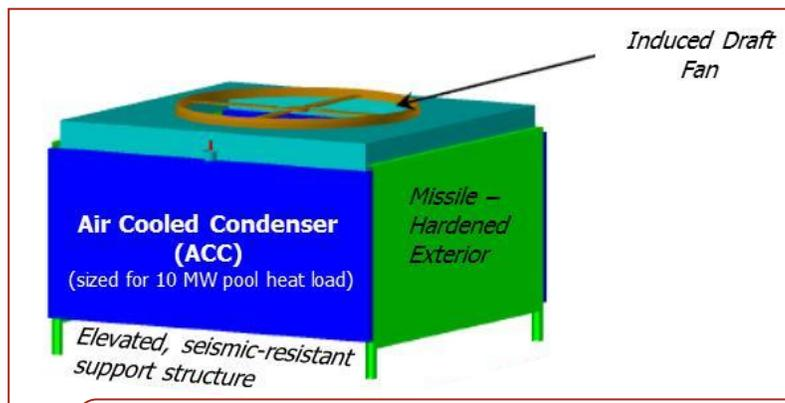
**Figure 2:** Air Cooled Condenser (ACC) Sized for 10 MW Pool Heat Load (disclosed to the U.S. patent office for international protection under application number 61475086)
