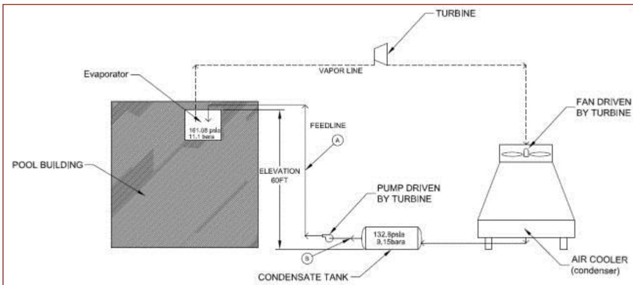
**Figure 1:** Process Flow Diagram of the HI-COOL System
