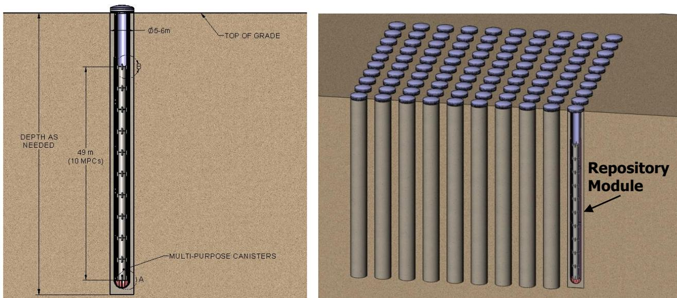
FIGURE 1: Cut-Away Views of Holtec's Modular HOMER Systems (left) and a Single Repository Module
