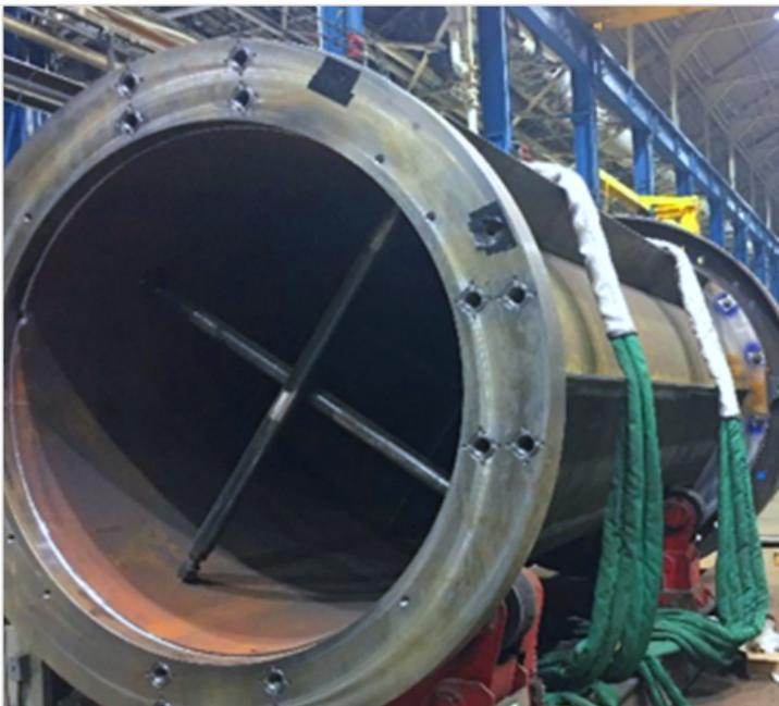
*HI-STAR 190 Transportation Overpack for Ukraine's Central Storage Facility under fabrication at Holtec*
