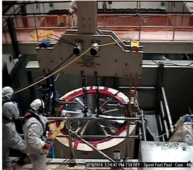
Holtec's HI-TRAC VW Transfer Cask and Luke Shipley, Radiation Protection Technician for TVA
