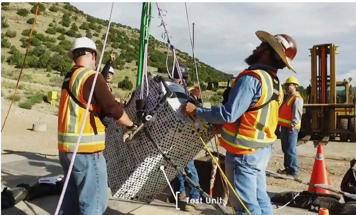
Crew Setting up the CG Over Corner Drop Test
