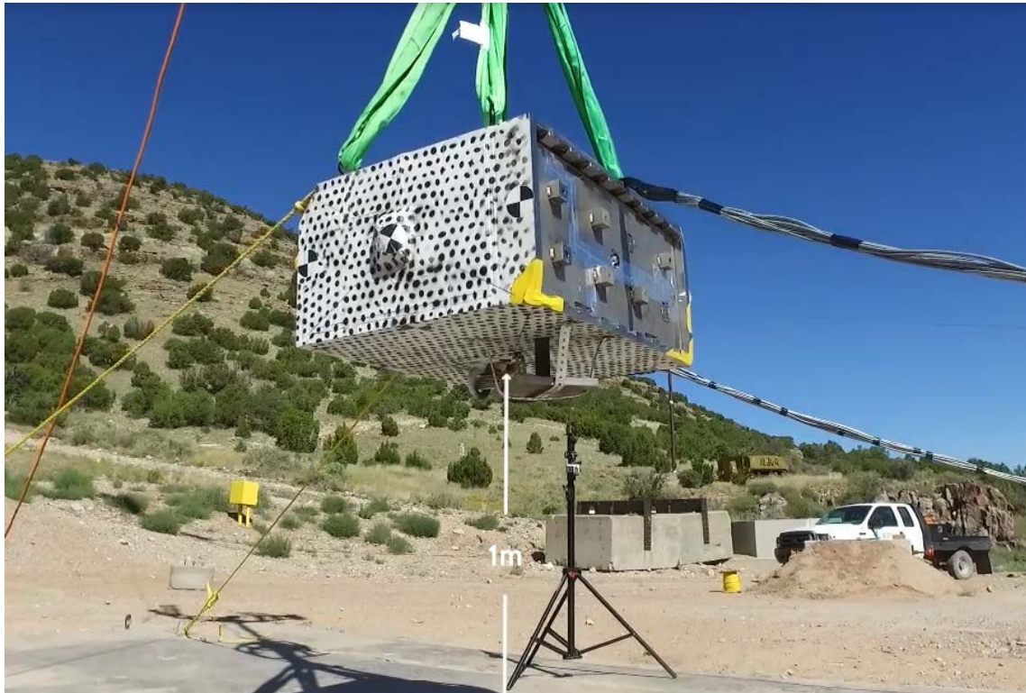
Test Set-up for the Puncture Drop
