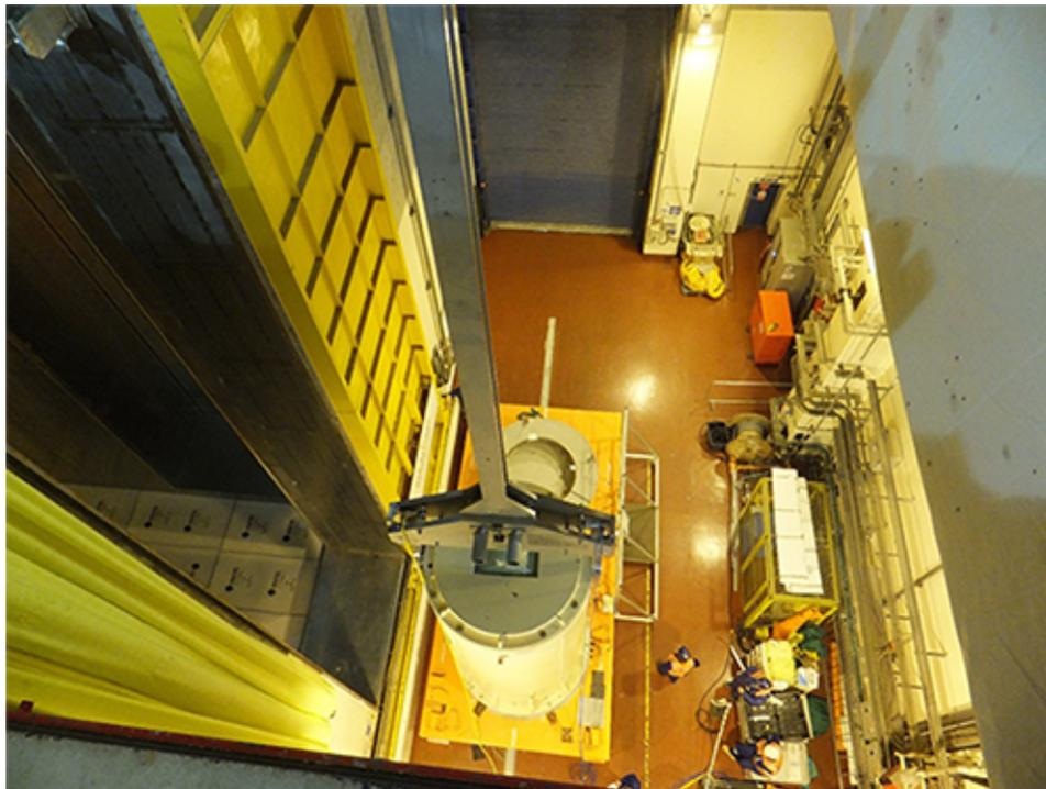
*HI-TRAC Transfer Cask Being Lifted into Flask Preparation Bay*
