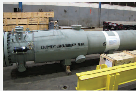
Two (2) Moisture Separator Reheater (MSR) Shell Drain Heat Exchangers for a PWR in Florida
