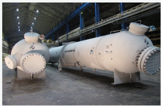
Two (2) Low Pressure Feedwater Heaters for a PWR in South Carolina
