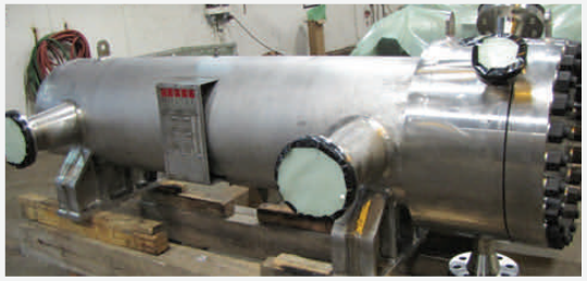
Sixteen (16) Reactor Cooling Pump Heat Exchangers for AP 1000 Nuclear Power Plants in China
