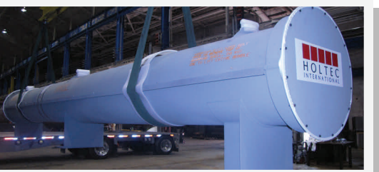
Two (2) Replacement Lube Oil Cooler Tube Bundles for a PWR in Florida
