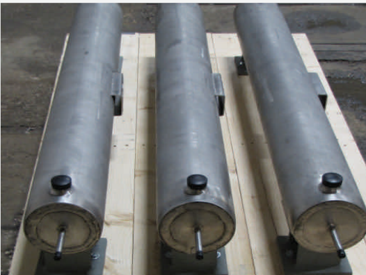
Three (3) Sampling Heat Exchangers with Helical Coil for a PWR in Slovenia
