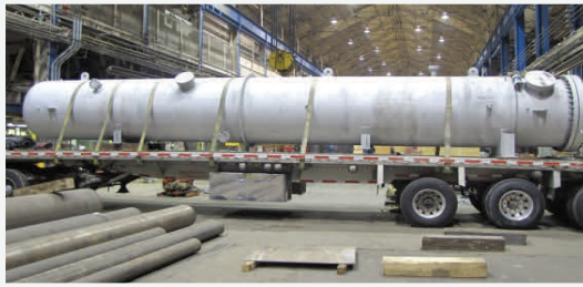
Six (6) Intermediate and High Intermediate Pressure Feedwater Heaters for a BWR in Minnesota
