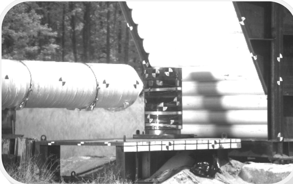
High Speed Photographs of Missile Approaching the Cask at 888 Ft/Sec Just Prior to Impact
