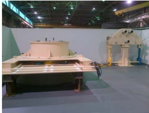
MPC Stack-up/Transfer Mock-up and Lift Yoke
